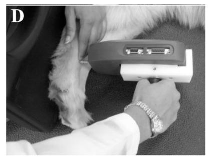
maximum force of the instrument was reached. Each dog was assigned a feasibility score that described the ease with which data could be collected per device; with scores ranging from 0 to 2 'easy data collection' and those from 3 to 5 'difficult data collection'. Dogs scoring higher than 2 did not return for the second evaluation and their data were excluded from analysis.
